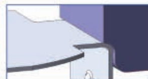
Add a Form Punch that Coins/Sets the Radius
