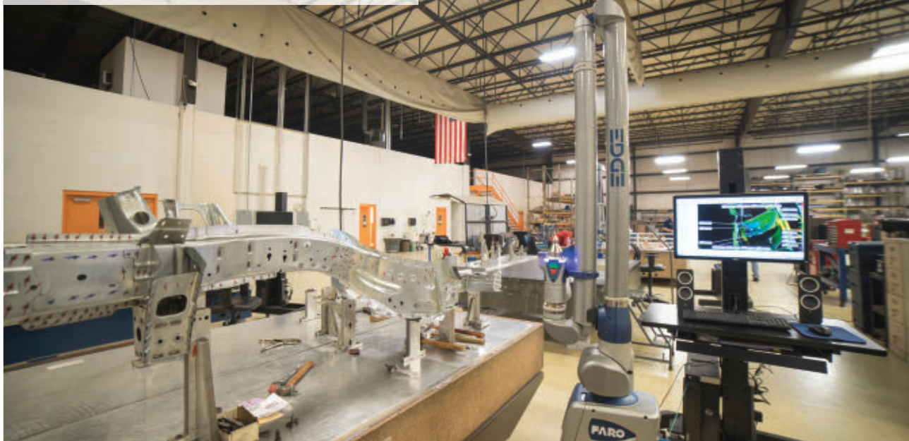
A Faro scanner scans a part and verifies part quality with customer data.
