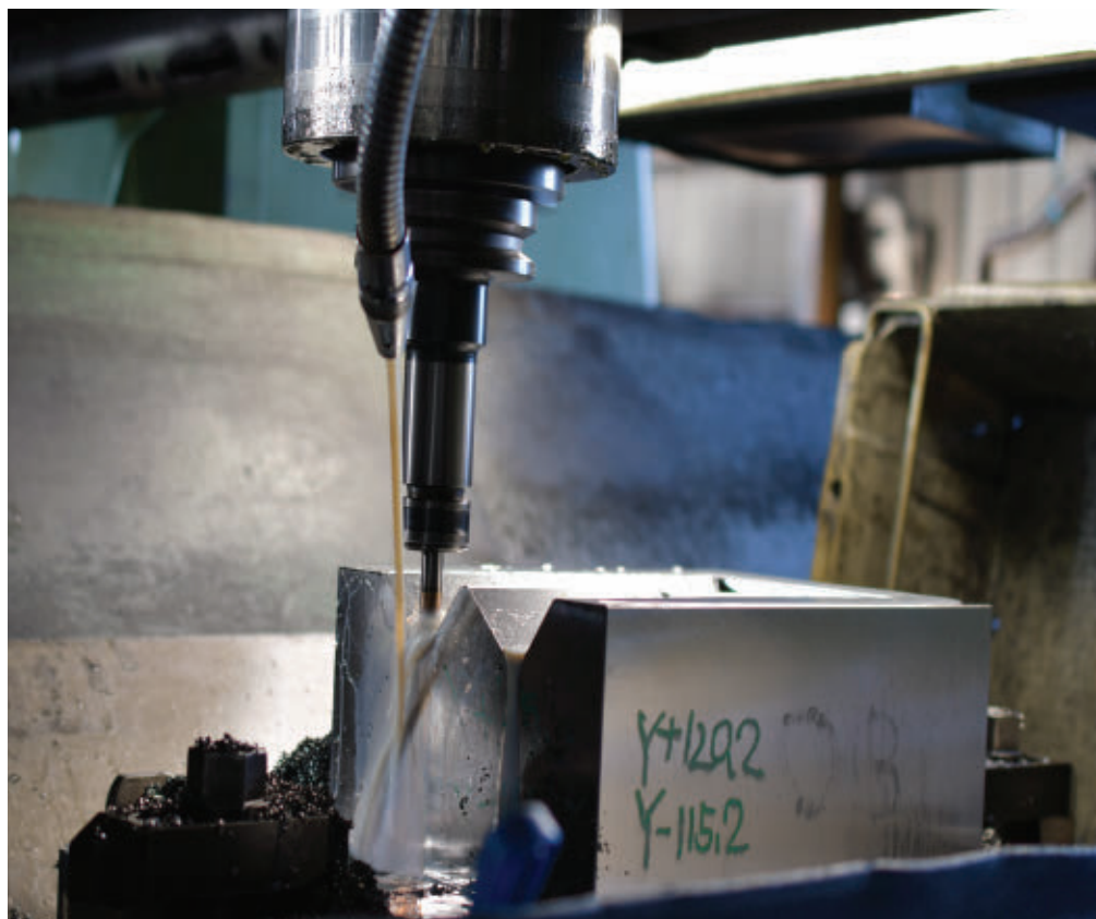
The die build milling and machining process creates combined metal scrap and fluid waste.
