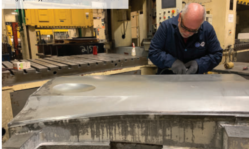
Large prototypes are formed in Kirksite tools.
