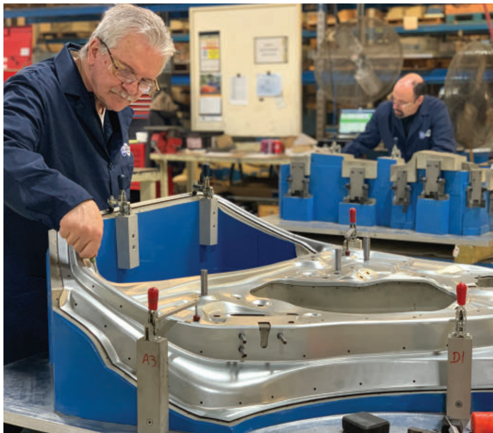
A highly skilled fabricator qualifies a part to ensure that it meets customer specifications. The nature of prototyping is such that there are times when each part needs a craftsman to fine-tune-shape it to specification by hand.
