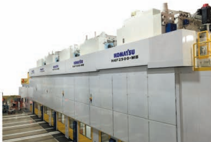
H4F 4-Point Servo Mechanical Press, 5-press tandem line; 4 lines installed at FCA plants in Michigan
