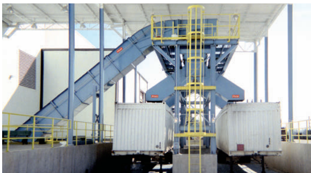
Loadout systems automatically transfer metal scrap into distribution containers for transport to a metal recycler. Level sensors alert operators and scrap dealers when the container is filled to capacity.
